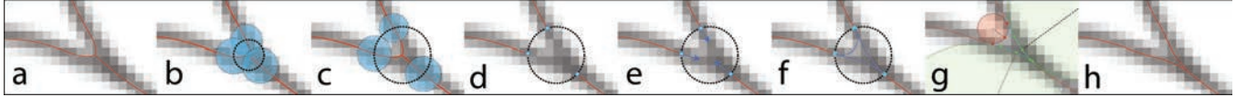
Fig. 7. Reverse drawing. For correct centerline estimation in the proximity of overlapping strokes (e.g., at junctions) (a), our algorithm first identifies the ambiguous region (b,c) and removes the corresponding centerline estimates (d). From the intersections of the ambiguous region with the base centerlines (e), continuous candidate centerlines ( CC_s ) are computed (e, f). Then the stroke curvatures of the CC_s are evaluated (g), and the final centerline configuration is selected (h).
